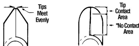
A precision tip interface assures clean cutting of fine wires, while the "no contact" area behind the tips extends cutter life by allowing the tips to continue to meet as they wear.
