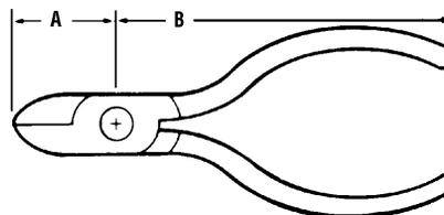
Leverage ratio is obtained by dividing dimension A into dimension B.
