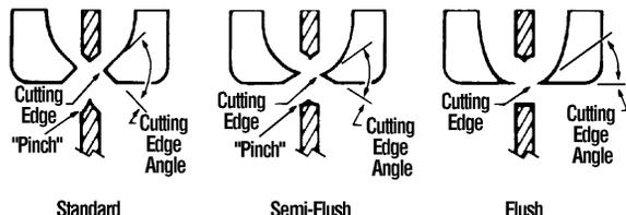
**Standard** cutting edges should be used for applications that are not sensitive to either the amount of shock transmitted through the wire to the component (during cutting) or to the amount of "pinch" left on the wire tip (after cutting).
